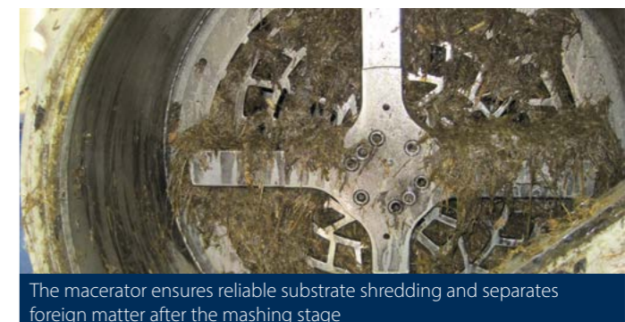
Mashing of the solid substrates already takes place in the first step
